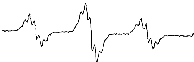
FIGURE 1 The e.s.r. spectrum of the 1,2,3,4-tetraphenylcyclopenta-1,3-diene radical anion in tetrahydrofuran at 203 K with lithium as the counterion
